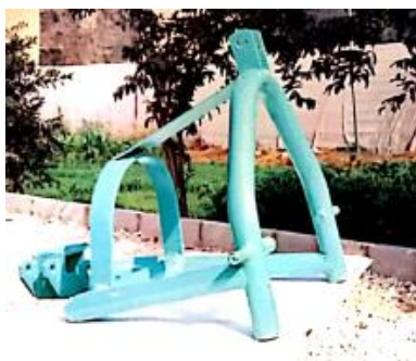
Figure 1. The frame and hitch points of olive harvester.
