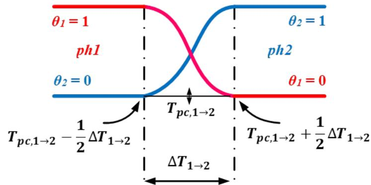
Figure 1. Modelling of phase change temperature transition interval [11]
