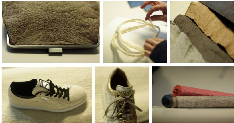
Şekil 8. Ananas yaprağı liflerinden üretilmiş 'Pinatex' isimli deri benzeri ticari malzeme ile üretilen ürünler [68, 127] (Commercial products such as 'Pinatex' produced from leather-like material which is derived from pineapple leaf fibers)
