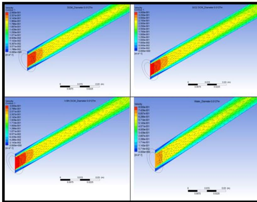
**Figure 10.** Velocity contours of the nanofluids and water in terms of pipe diameter (d=0.0127m=1/2")
