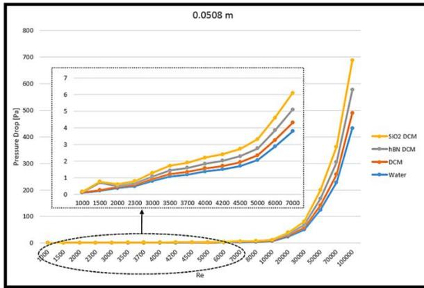
**Figure 8.** The alteration of pressure drop for increasing Reynolds numbers at 0.0508 m diameter
