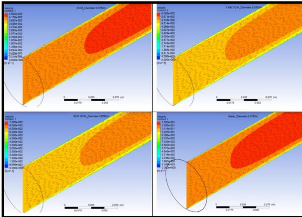
Figure 14. Velocity contours of the nanofluids and water in terms of pipe diameter ( $d=0.0762m=2\frac{1}{2}''$ )
