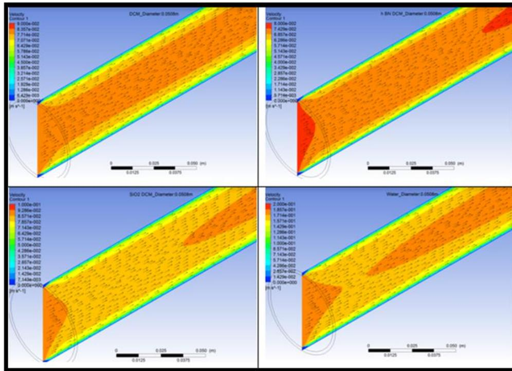
Figure 13. Velocity contours of the nanofluids and water in terms of pipe diameter ( $d=0.0508m=2''$ )
