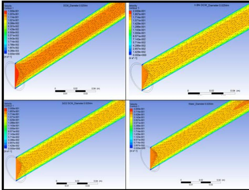
**Figure 11.** Velocity contours of the nanofluids and water in terms of pipe diameter ( $d=0.0254m = 1''$ )
