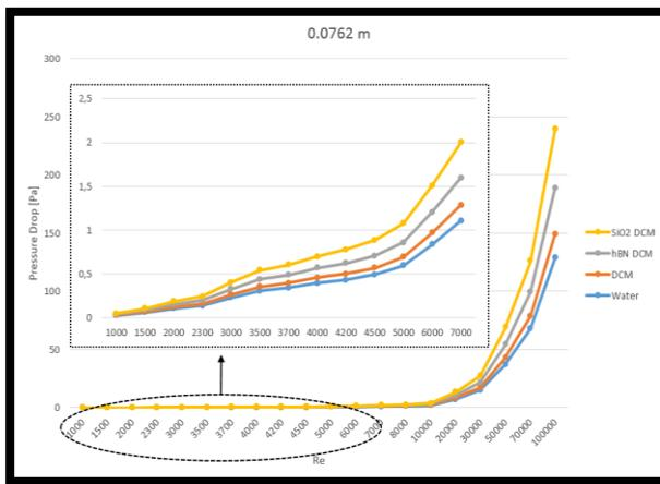
**Figure 9.** The alteration of pressure drop for increasing Reynolds numbers at 0.0762 m diameter
