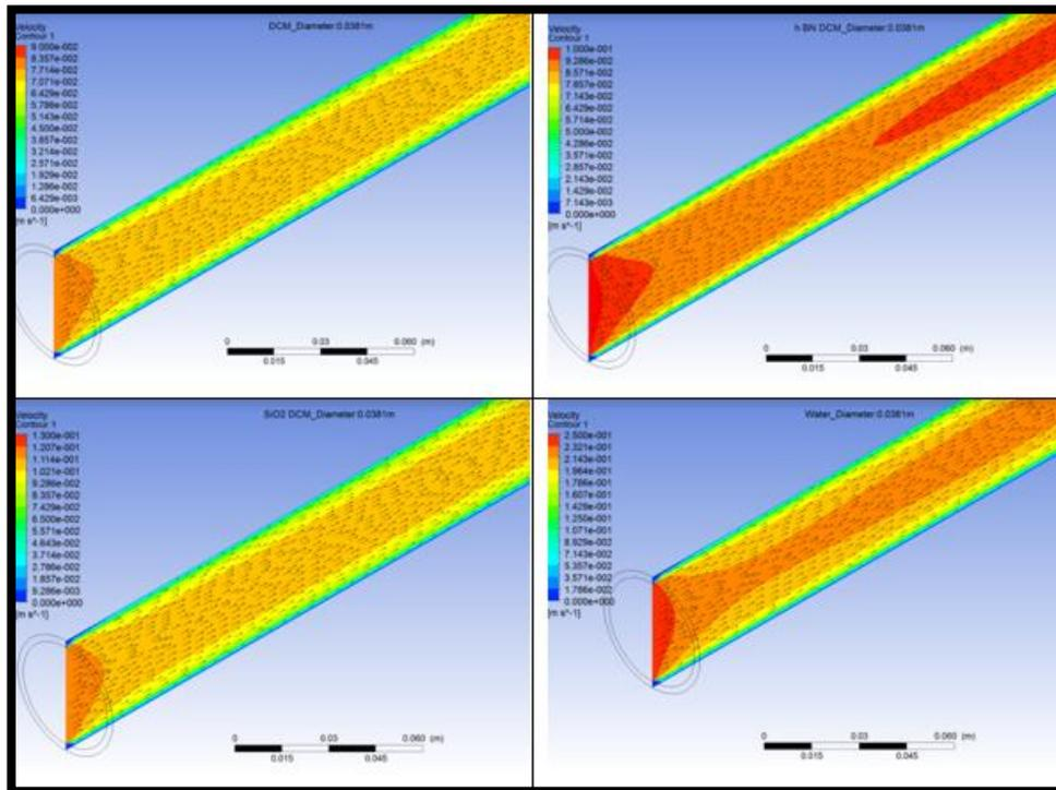
**Figure 12.** Velocity contours of the nanofluids and water in terms of pipe diameter ( $d=0.0381m = 1\frac{1}{2}''$ )
