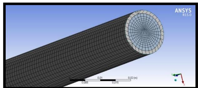
**Figure 2.** The generated solution grid
