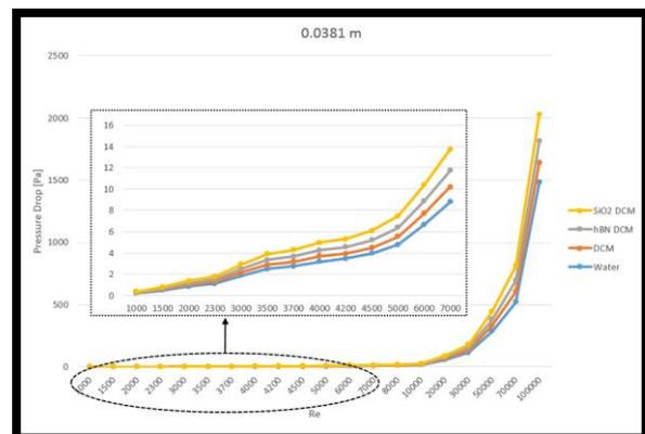
Figure 7. The alteration of pressure drop for increasing Reynolds numbers at 0.0381 m diameter
