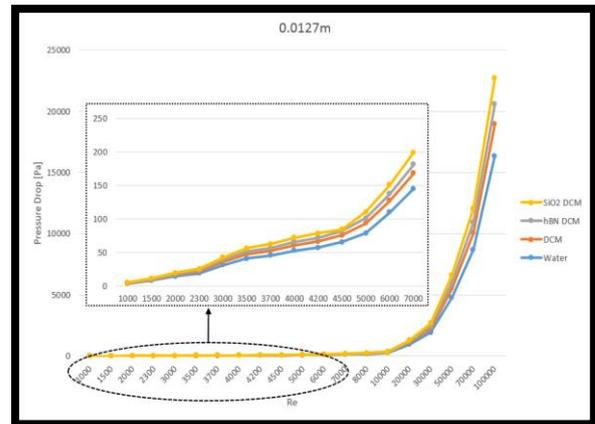
Figure 5. The alteration of pressure drop for increasing Reynolds numbers at 0.0127 m diameter
