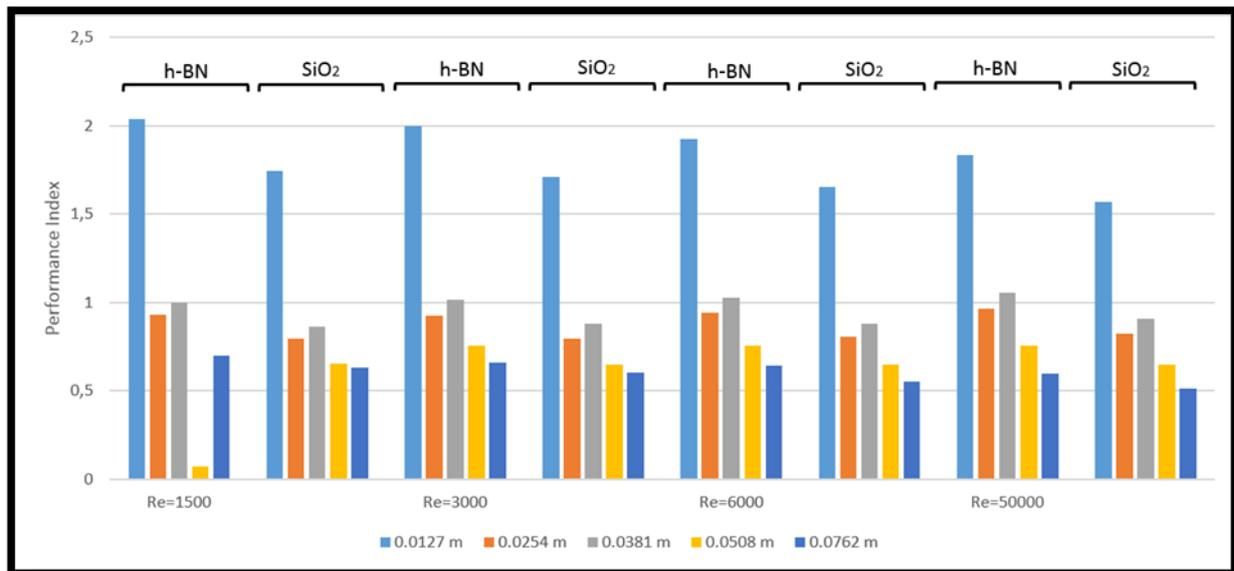
**Figure 15.** Performance index of nanofluids depending on Reynolds number for various diameters
