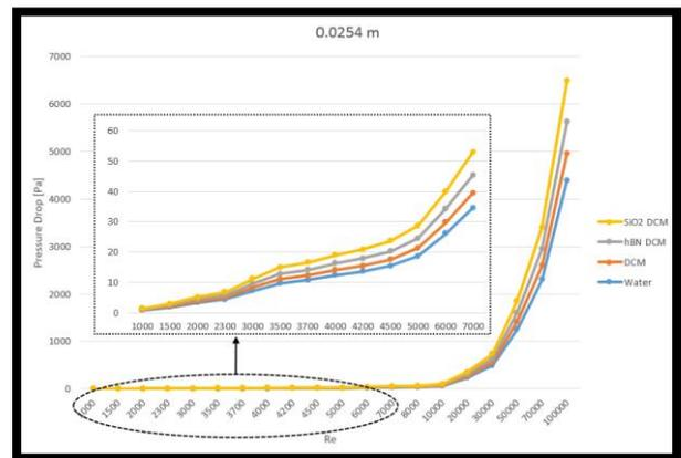
Figure 6. The alteration of pressure drop for increasing Reynolds numbers at 0.0254 m diameter
