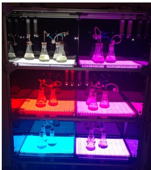
**Figure 1.** Arduino based computer controlled addressable RGB LED light system used for the experiments.
