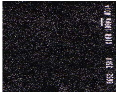
Fig.6 X-ray map of Samp. 9 Aluminum glaze
