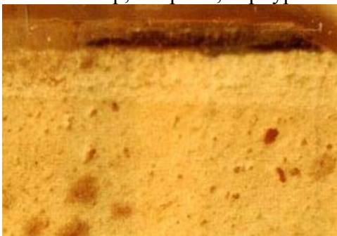
Fig.3 Thin sec. photo of texture, glaze+slip with dye and body, and poros are also seen
