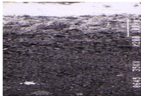
Fig.14 SEM mic.grph., Samp. 11, glaze+slip+body, finer quartz particles with interstitial glass
