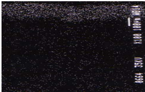
Fig.12 X-ray map of Samp. 9 Lead, glaze+slip+paste
