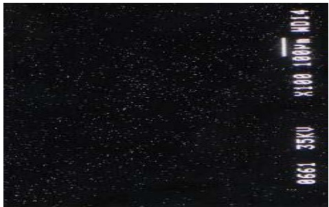
Fig.11 X-ray map of Samp. 9 Magnesium
