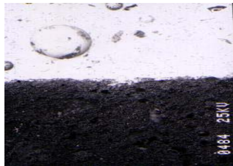
Fig.4 SEM mic.graph.,Samp.7 Coloured glaze brick piece
