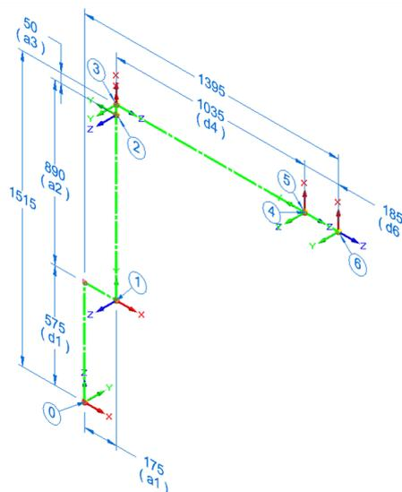
**Figure 2.** Schematic of robot shown at Figure 1
