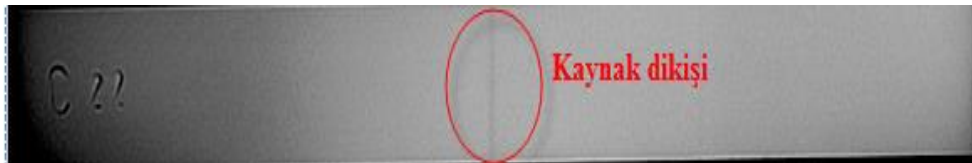
Şekil 1. Radyografik muayene test numunesi (Figure 1. Radiographic image of laser welded sample)
