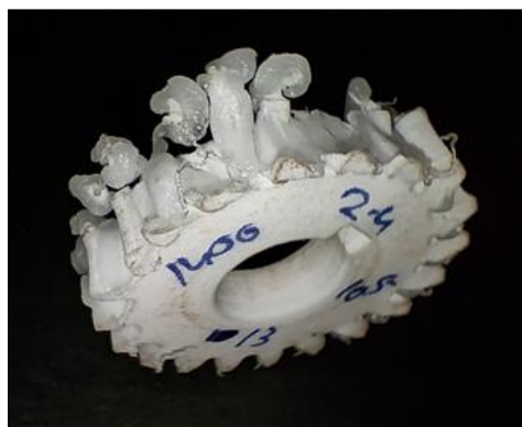
Figure 9. Failure of spur gear
