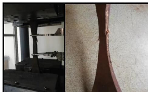
Figure 12. Tensile test image of the unspliced belt
