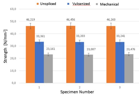
Figure 17. Comparison of strength of belt splicing methods
