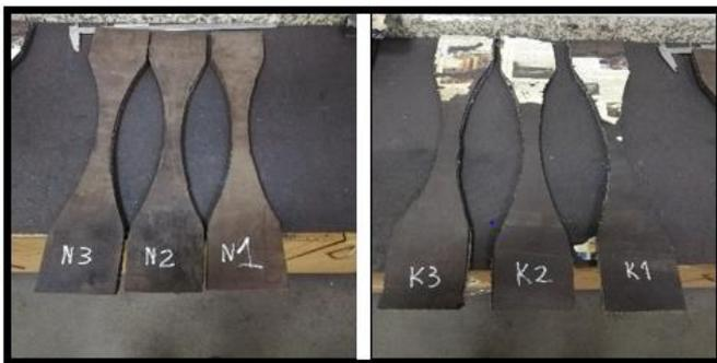
Figure 7. Bowtie-shaped specimens: Original unspliced (N coded) and vulcanized (K coded) belt specimens.
