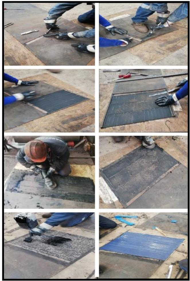
**Figure 4.** Images of belt splice preparation stages
