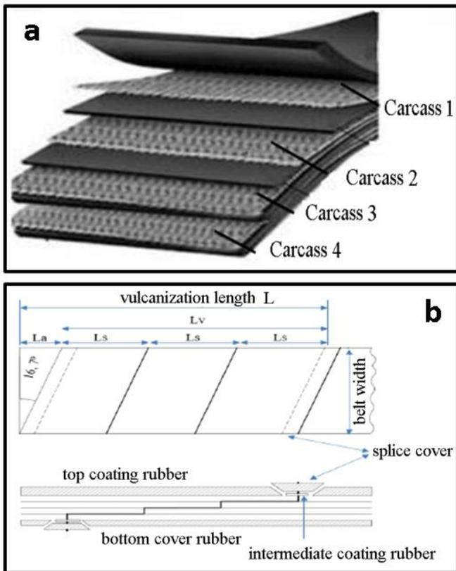
**Figure 3.** Schematic representation of four-layer carcass belt (a) and belt splice (b) [8, 17]
