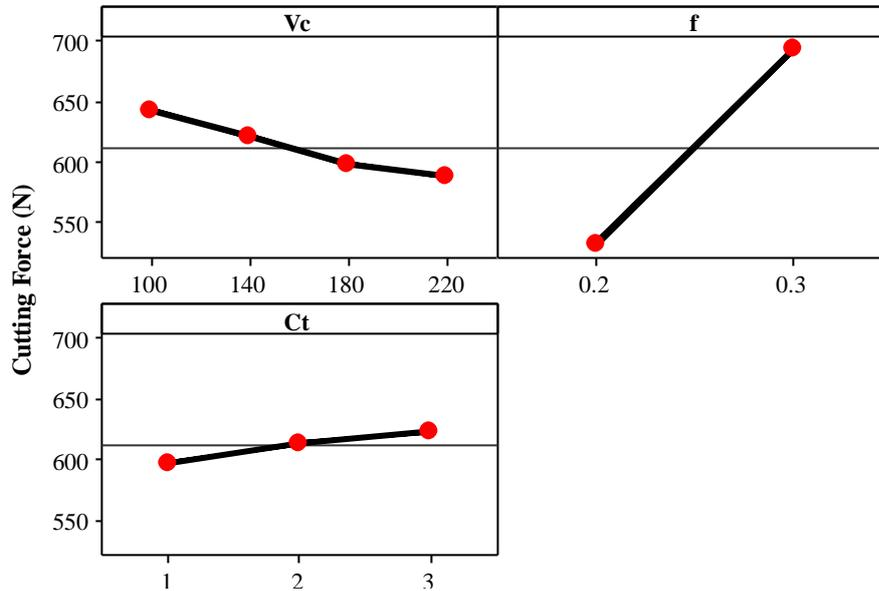
Figure 4. The effect of cutting parameters and coating materials on the cutting forces
