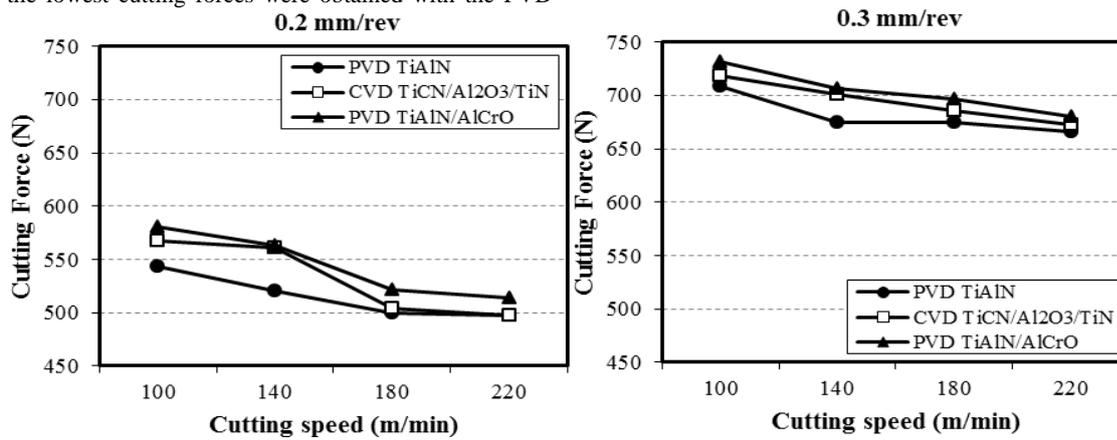
Figure 2. The variation of cutting forces between the three tools depending on the cutting speed and feed rate
