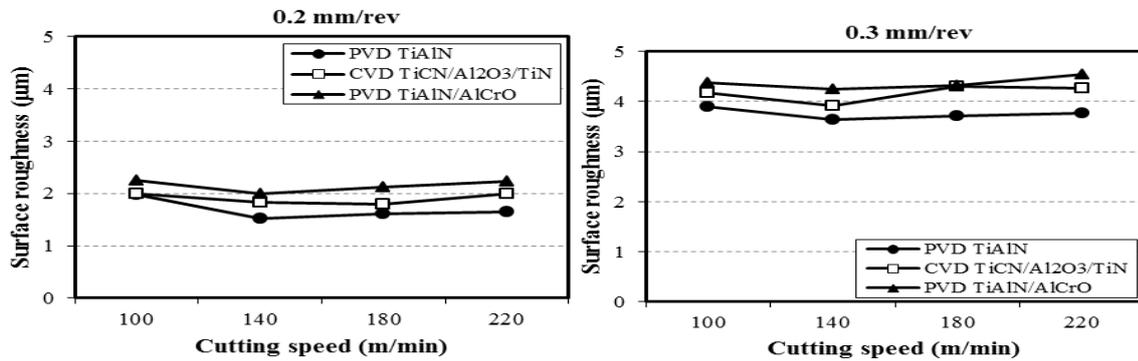
Figure 3. The variation of surface roughness between the three tools depending on the cutting speed and feed rate
