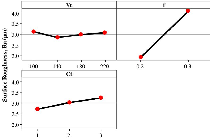
Figure 5. The effect cutting parameters and coating materials on the surface roughness
