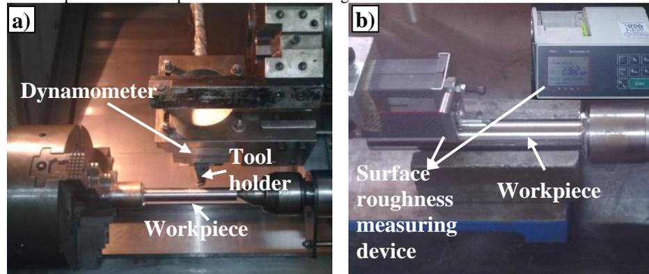
**Figure 1.** Experimental configuration for measuring of a) cutting force and b) surface roughness
