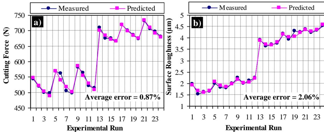
Figure 6. The relation between the values measured during the test and the estimated values a) cutting force, b) surface roughness
