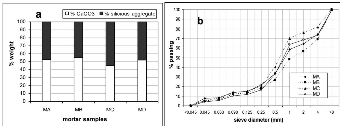
Fig. 7 [a] Aggregate/binder ratio of mortars, [b] grain size distributions of the aggregates
