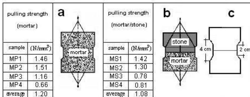
Fig. 12 [a] Mortar, [b,c] mortar/stone pulling test apparatus, and results
