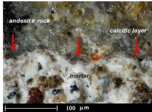
Fig. 13. Secondary calcite layer formation between andesite aggregate and binder
