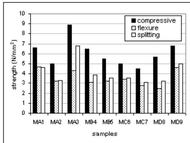
Fig. 11 Mechanical properties of the mortars
