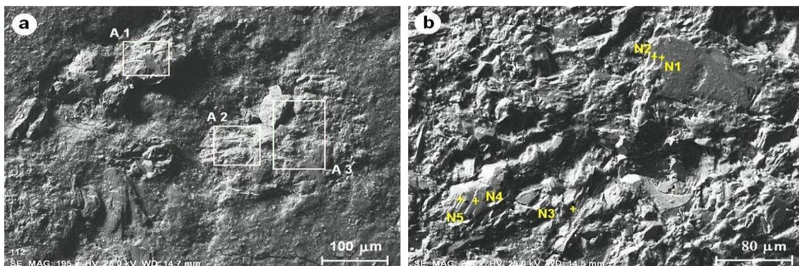
Fig.14 [a] SEM photos and [b] EDS (area and points) analysis of mortar samples.
