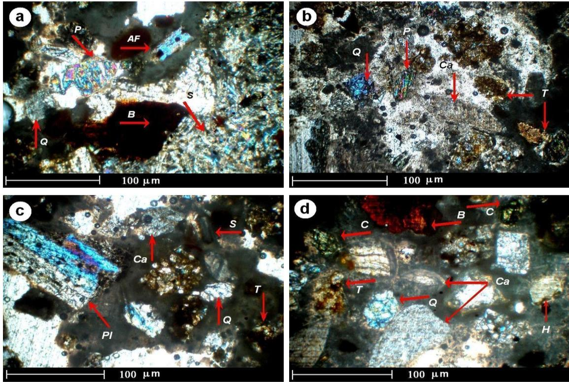
Fig. 8 [a,b,c,d] Thin section view (double nicols) of mortars and their minerals (Ca: calcite, B: biotite, Q: quartz, Pl: plagioclase, P: pyroxene, AF: alkaline feldspar, S: sanidine, C: chlorite, H: hornblend, T: tuffic pieces.
