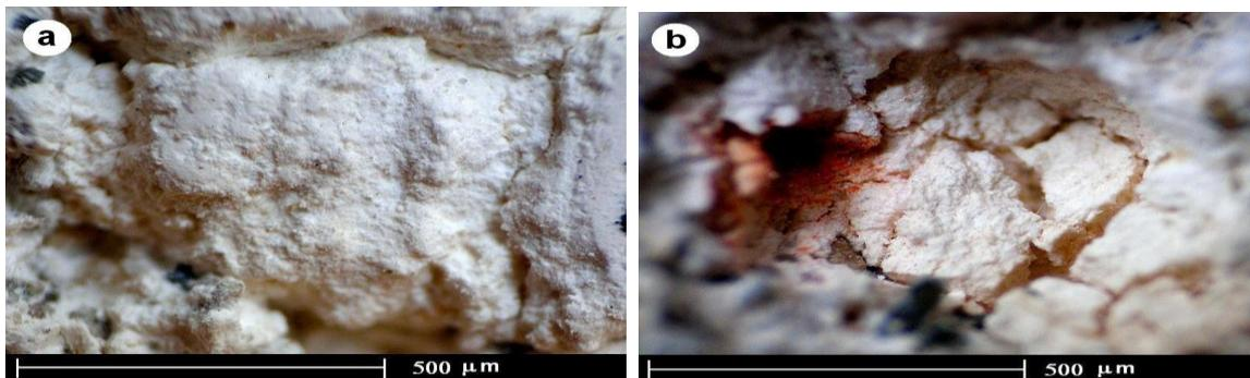
Fig. 6 Lime lumps in the mortar, [a] pure CaCO<sub>3</sub>, [b] lime lump shrinkage cracks
