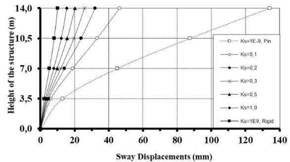
Figure 14. In the example problem, the spring constants ( $K_s$ ) and height of the structure
