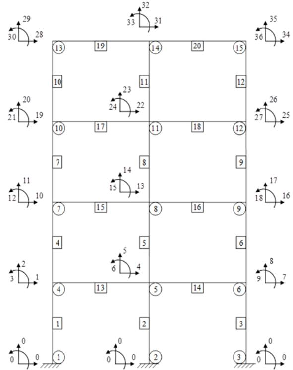
Figure 11. Coding of joints and numbering of members
