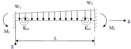
Figure 7. A linearly distributed load exposed to a beam with semi-rigid end connections
