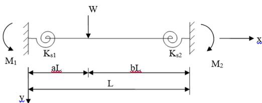
Figure 6. An unsymmetrical point load exposed to a beam with semi-rigid end connections
