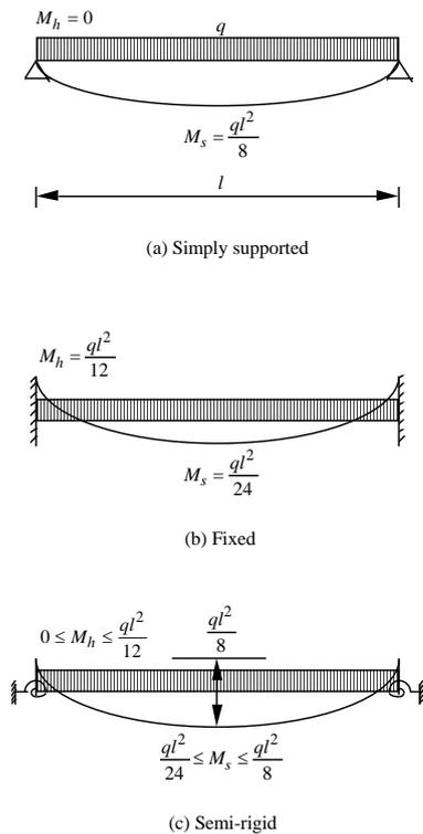
Figure 3. Beam with various end conditions [1]
