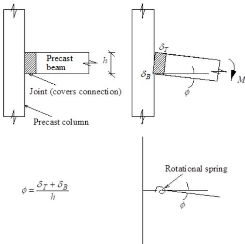
Figure 1: Simplified definition of joint rotation [1]
