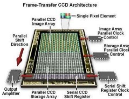
**Figure 1.** Frame Transfer CCD Architecture [6].
