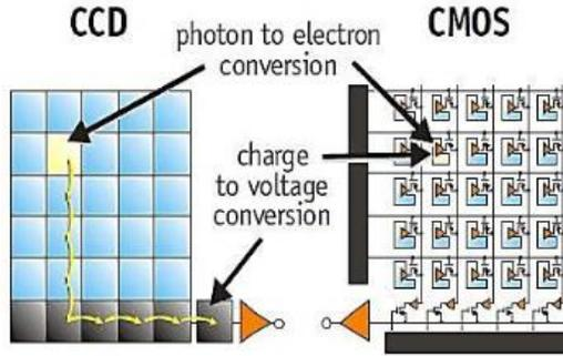
Figure 3. Working differences of CMOS and CCD [11].
