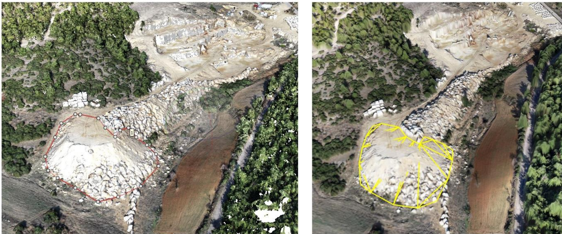
Şekil 6. Hacim hesabı yapılan pasa alanı. Agisoft Metashape (sol), Virtual Surveyor (sağ) (The area of the passage for which the volume is calculated. Agisoft Metashape (left), Virtual Surveyor (right))
