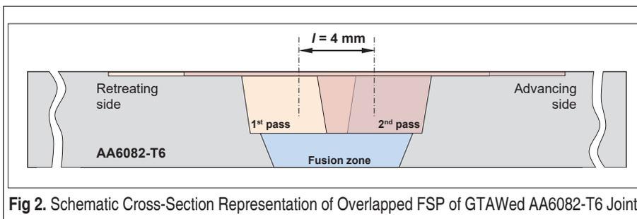
**Fig 2.** Schematic Cross-Section Representation of Overlapped FSP of GTAWed AA6082-T6 Joint
