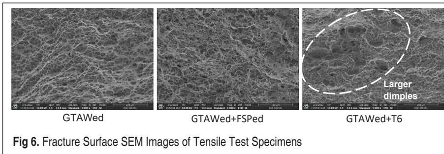
**Fig 6.** Fracture Surface SEM Images of Tensile Test Specimens
