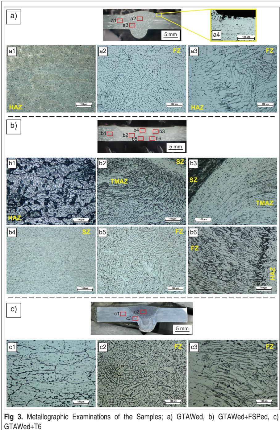
**Fig 3.** Metallographic Examinations of the Samples; a) GTAWed, b) GTAWed+FSPed, c) GTAWed+T6
