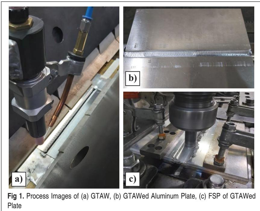
**Fig 1.** Process Images of (a) GTAW, (b) GTAWed Aluminum Plate, (c) FSP of GTAWed Plate
