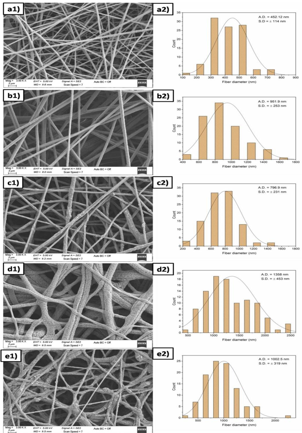
**Figure 2.** SEM micrographs of electrospun webs a1) PLA, b1) PLA-PVP, c1) PLA-PVP/ $\text{CaCO}_3$ , d1) PLA-PVP/MPEO, e1) PLA-PVP/ $\text{CaCO}_3$ /MPEO (Magnification: 3 kX, scale; 2  $\mu\text{m}$ ) and fiber diameters (a2-e2)
