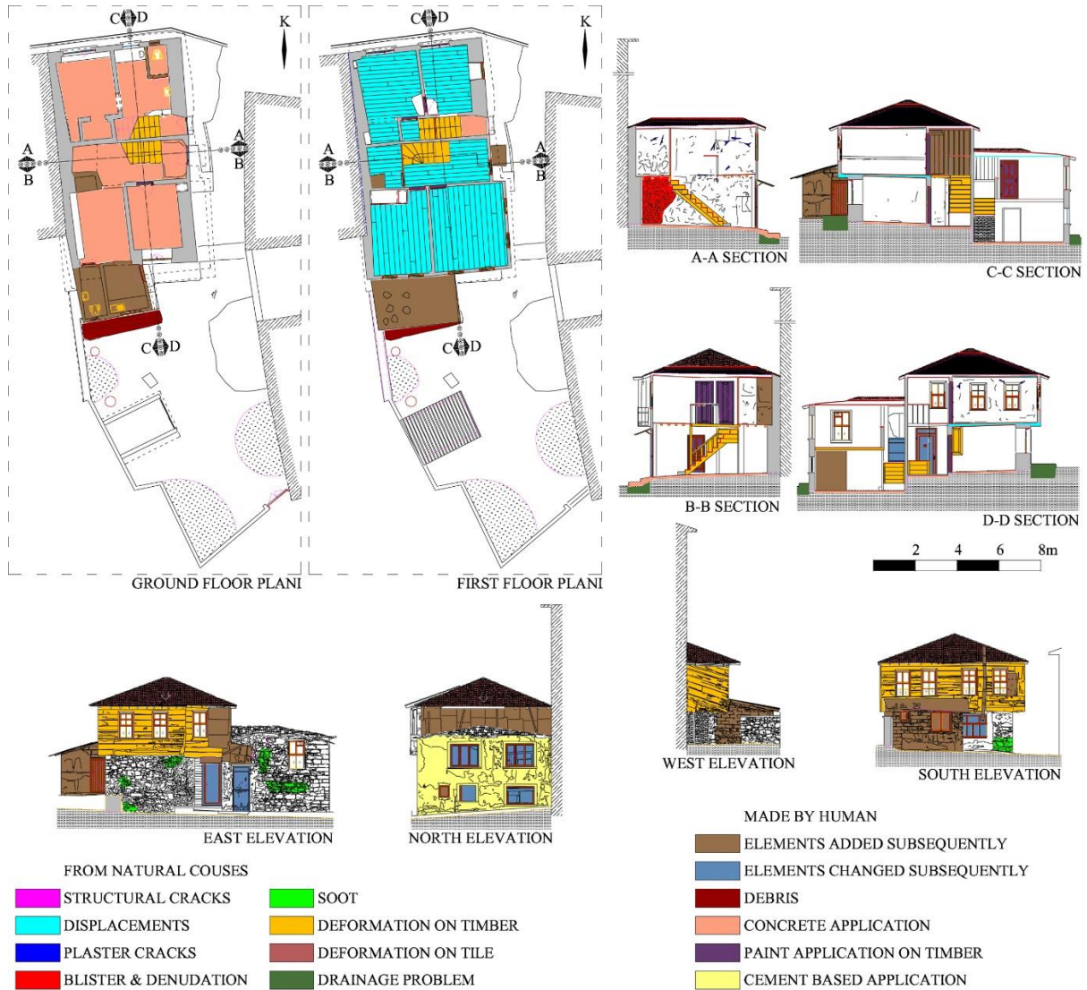
Figure 5. Deteriorations and corruptions
