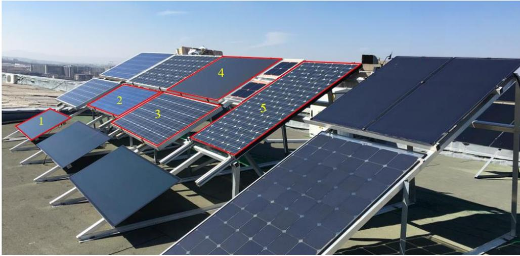
**Figure 1.** Configuration of ODTÜ-GÜNAM outdoor test facility (a) and tested modules – 1: CIS, 2: Poly-Si, 3: Mono-Si, 4:  $\mu$ c-Si/a-Si, 5: HIT (b)
