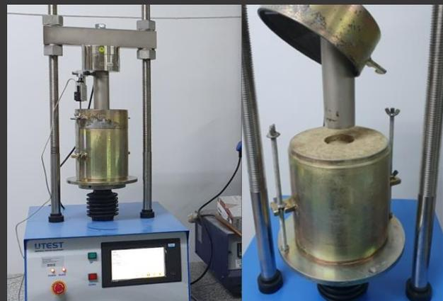
Figure 3. Automatic CBR test machine
