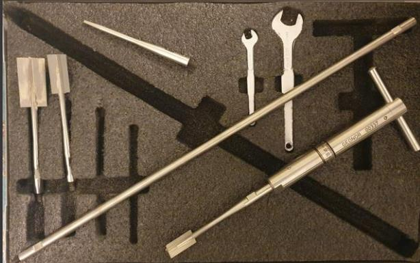
Figure 4. Hand vane shear tester
