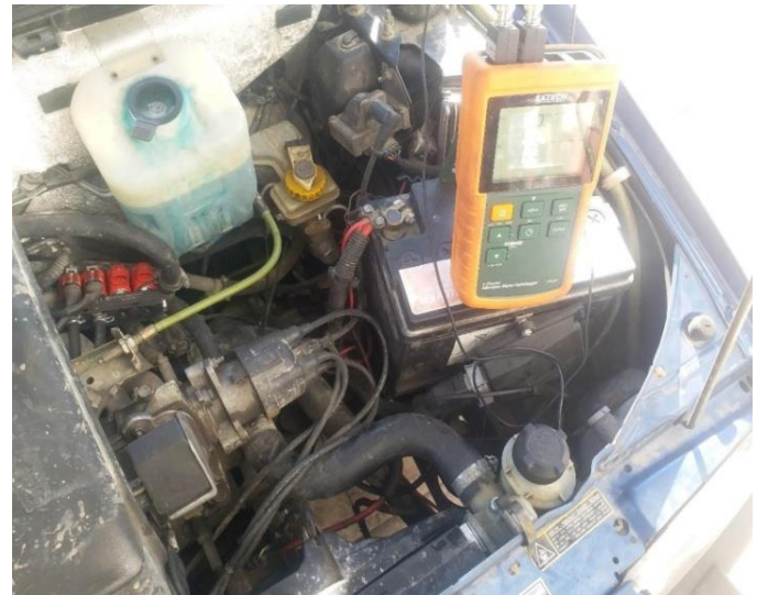
Fig. 1. Experimental Setup for Vibration Measurement of the Engine
