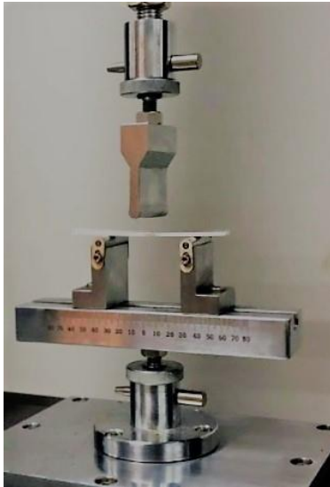
Figure 5. Bending test device.
