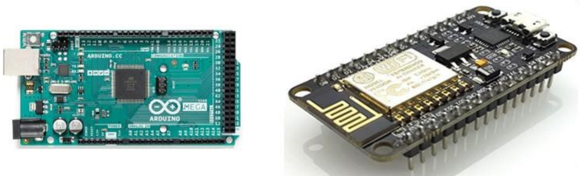
Figure 8. Arduino Mega 2560 (a) and NodeMCU ESP8266 (b)
