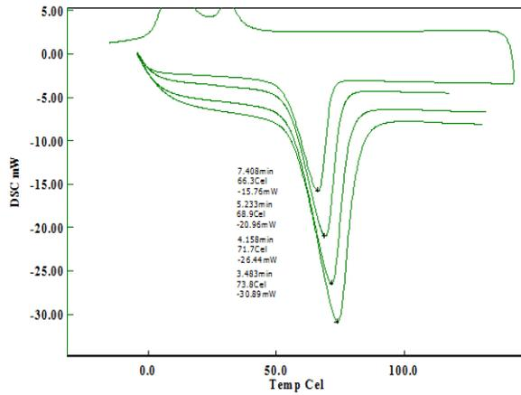
Fig.2. DSC curves of different heating rate for as-cast sample.
