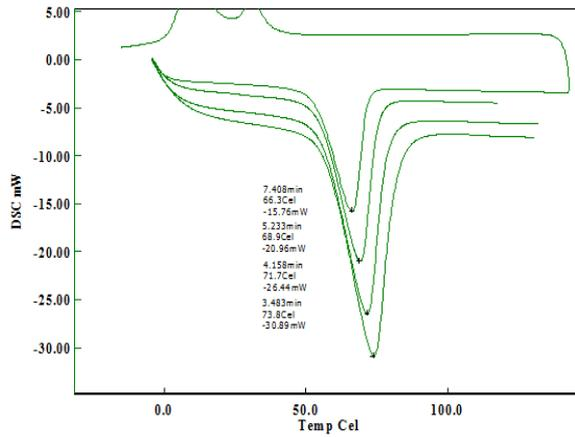
Fig.2. DSC curves of different heating rate for as-cast sample.
