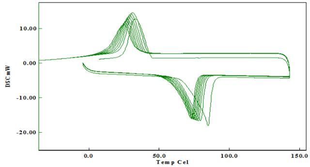
Fig. 4. The thermal cycles of DSC curves of heat treated sample at 800 C.
