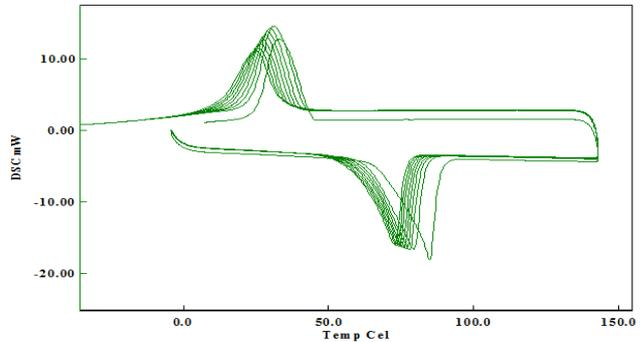
Fig. 4. The thermal cycles of DSC curves of heat treated sample at 800 C.
