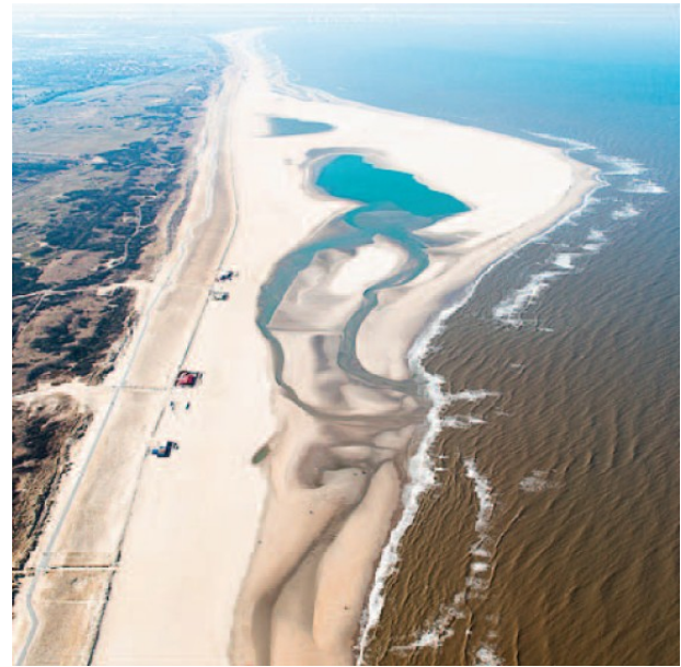
Şekil 2. Hollanda’da 2011 yılında yapılan mega besleme projesi (Mega nourishment project in Netherlands, which was built in 2011)
