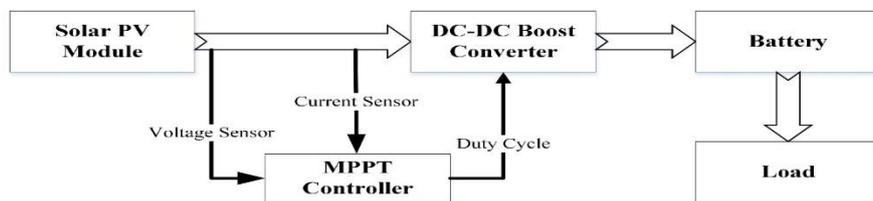
Figure 1. Block diagram of a PV system with MPPT controller
