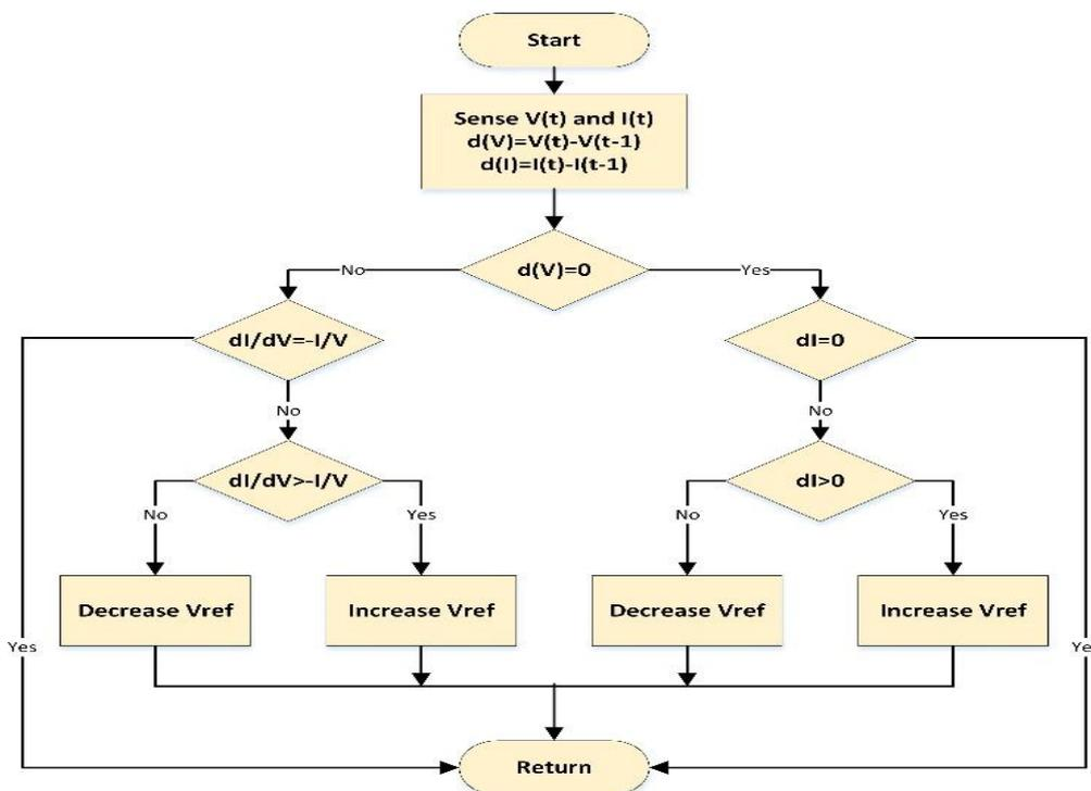
Figure 3. Flowchart of IC MPPT technique
