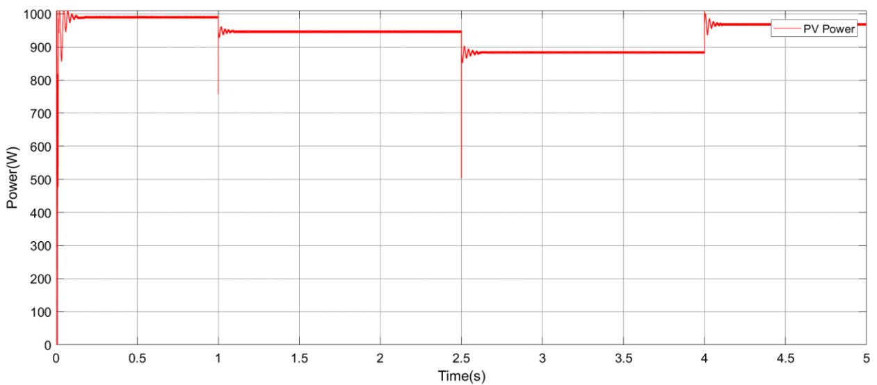
**Figure 10.** PV panel output power with IC for different temperature levels at constant irradiance
