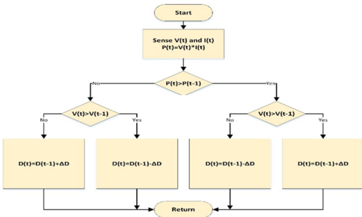
Figure 2. Flowchart of IC MPPT technique
