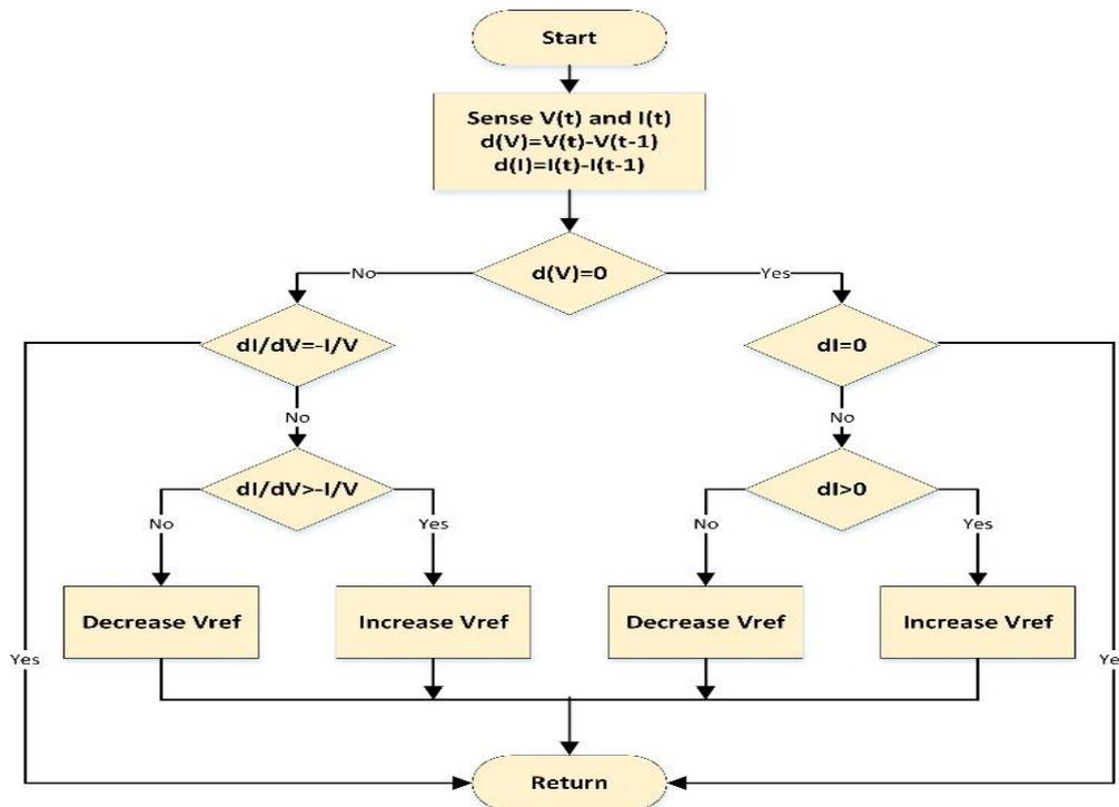
**Figure 3.** Flowchart of IC MPPT technique
