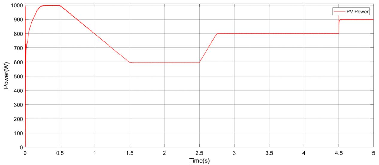
Figure 7. PV panel output power with P&O for different irradiance levels at constant temperature
