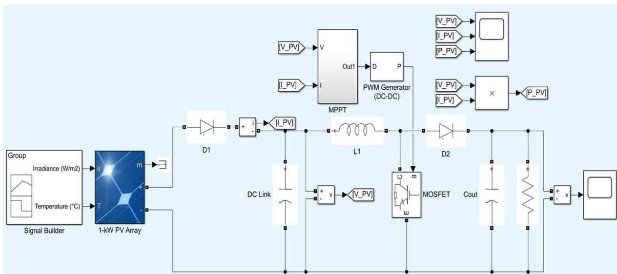
**Figure 4.** 1 kW PV array and DC-DC boost converter with MPPT controller
