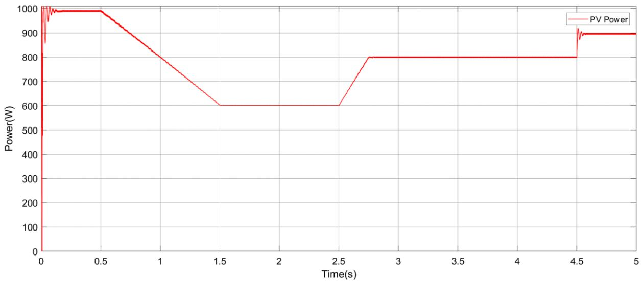
**Figure 9.** PV panel output power with IC for different irradiance levels at constant temperature
