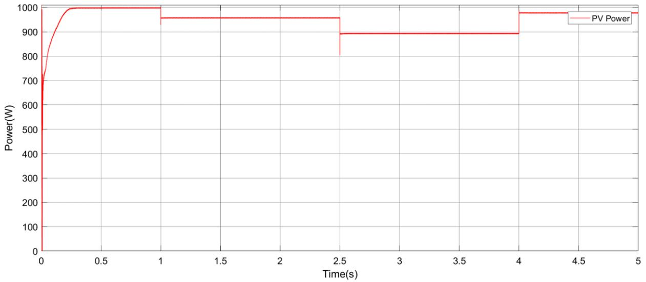
**Figure 8.** PV panel output power with P&O for different temperature levels at constant irradiance
