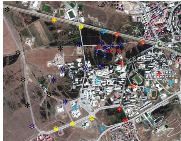
Figure 3. The distribution of night sky-brightness values at Ataturk University campus. The measured points are colored according to level of sky-brightness based on Table 2. The results were obtained from an average of measurements taken from four different nights.
