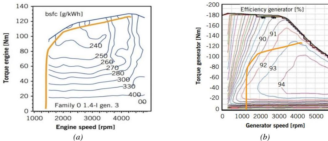
Figure 6. The specific fuel consumption map of the (a) ICE and (b) generator characteristics [22].
