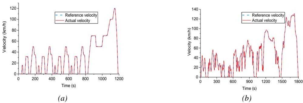
Figure 11. Reference and actual velocities of (a) NEDC simulation, and (b) WLTC simulation.
