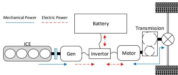
Figure 1. The structure of the series hybrid electric vehicle.
