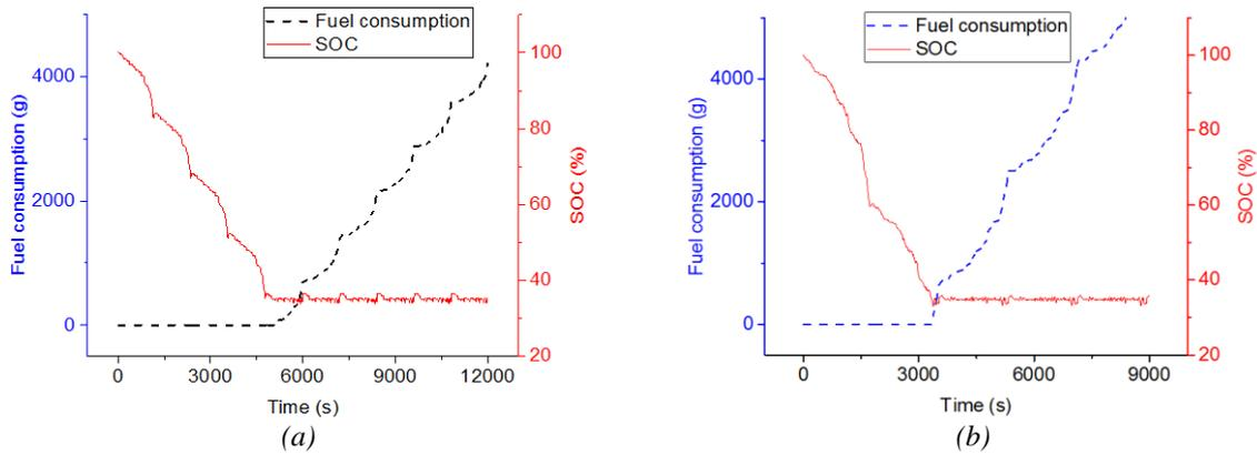
Figure 13. Fuel consumptions and SOC of (a) NEDC simulation, and (b) WLTC simulation, respectively.
