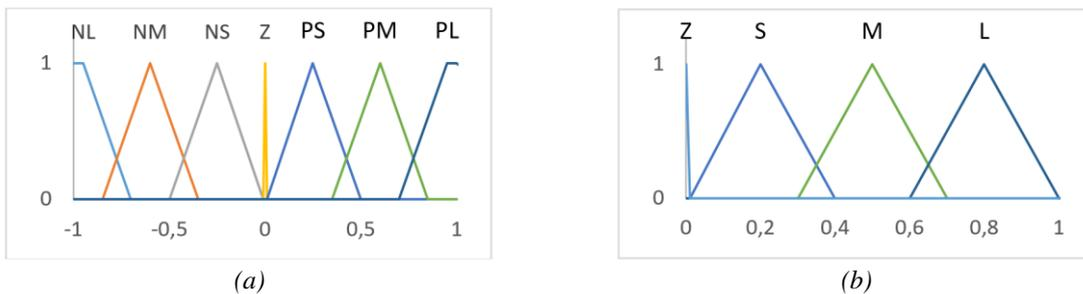
Figure 9. Membership functions of (a) ICE/generator power change output and (b) regenerative braking output, respectively.
