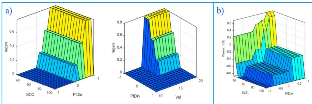
Figure 10. Surface view of the rules for a) regenerative braking, b) the ICE power change.
