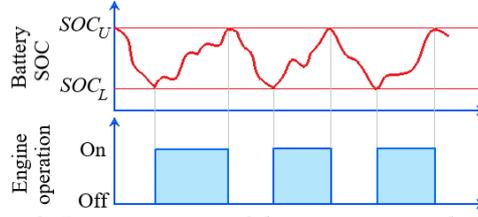
Figure 2. Demonstration of thermostat control method.
