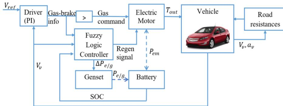
Figure 4. Schematic of the model used in the simulation.
