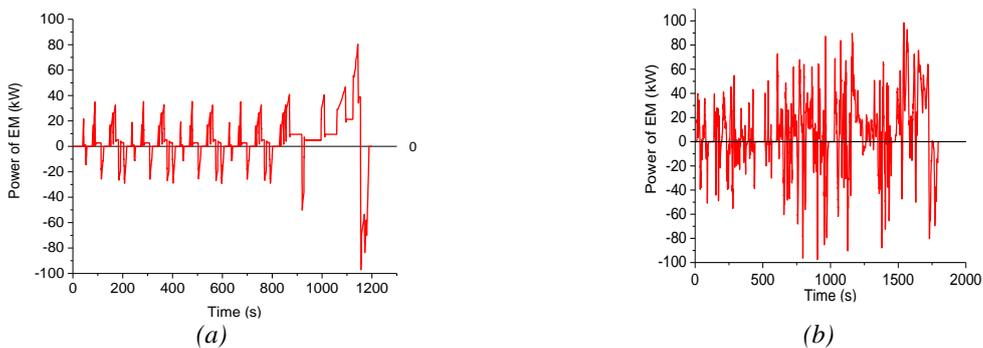
Figure 12. Electric motor power change in (a) NEDC simulation, and (b) WLTC simulation.
