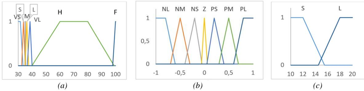
Figure 8. Membership functions of (a) SOC, (b) driver, and (c) velocity inputs, respectively.
