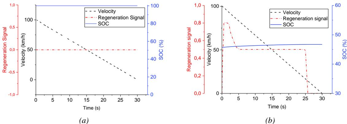
Figure 14. Regenerative braking, when the SOC is (a) very high, and at (b) lower SOC levels.
