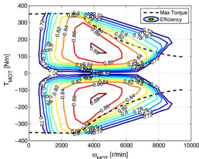
Figure 5. EM torque and efficiency curves [20].
