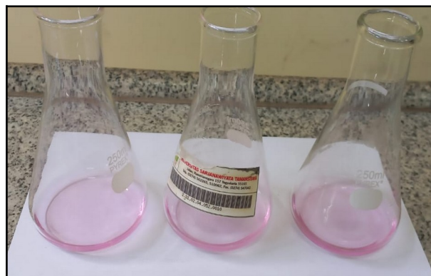
Figure 4: The addition of phenolphthalein indicator produced a pink color at the end of the alkalimetric titration of a weak acid with a strong base.
