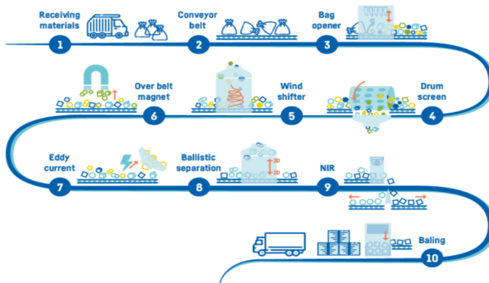
Figure 1. Sorting Process for Packaging Waste (Pietrelli et al., 2017).
