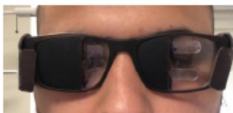
Figure 5. Visual field testing with Peli prism attached to simulation goggles
