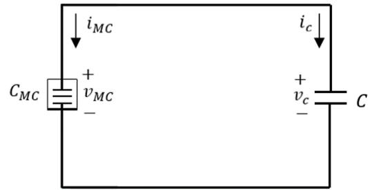
Figure 3. The memcapacitor-the LTI capacitor circuit examined in [48].
