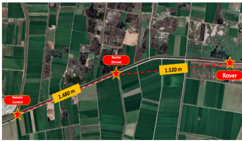
Fig. 18. Open Area (Rural) Communication Test Result.
