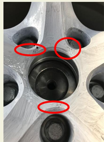
Figure 19. 4.000.000 cycles in long test
