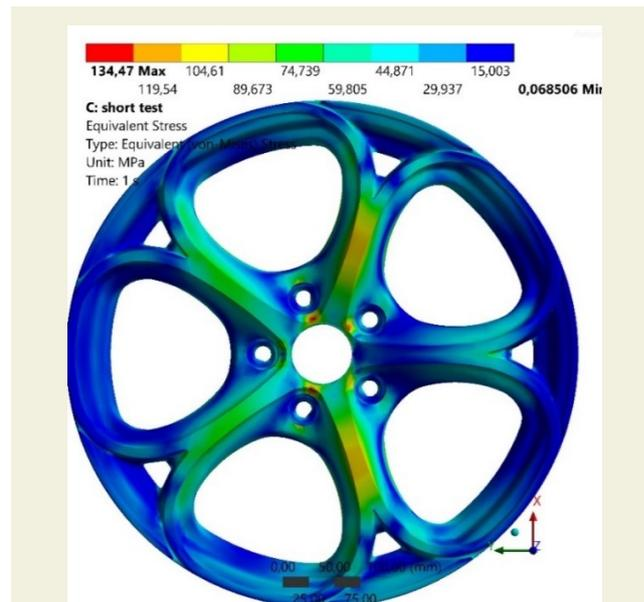
Figure 7. Maximum equivalent stress, short test
