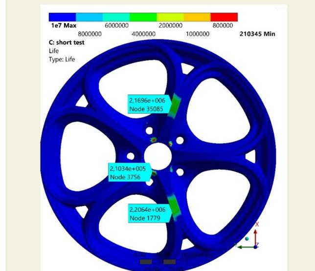
Figure 9. Fatigue life in short test
