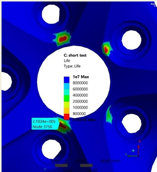
Figure 11. Fatigue life detail in short test
