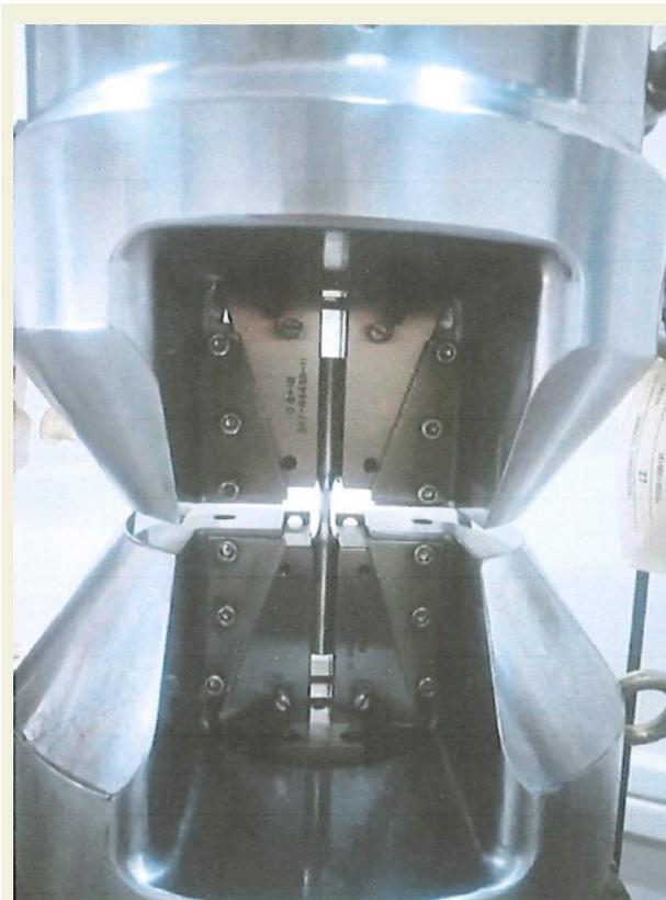
**Figure 3.** Testing configuration and fatigue specimen in testing
