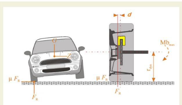
Figure 6. Bending fatigue representational image
