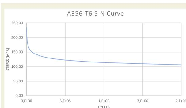
**Figure 4.** S-N curve of A356-T6 wheels
