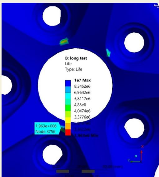
Figure 12. Fatigue life detail in long test
