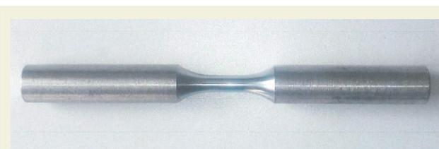
**Figure 2.** Fatigue specimen of Döktaş
