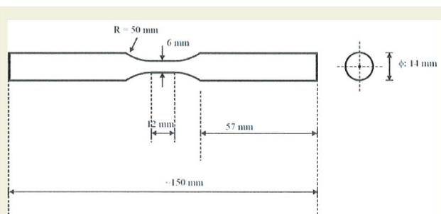
**Figure 1.** Dimensions of Döktaş Fatigue specimens acc.to ASTM E466
