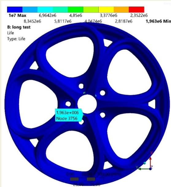
Figure 10. Fatigue life in long test
