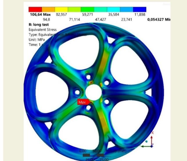
Figure 8. Maximum equivalent stress, long test
