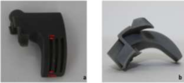
Figure 4. 3D printed suction-insert for compact three-rovings yarn a) front view b) side view
