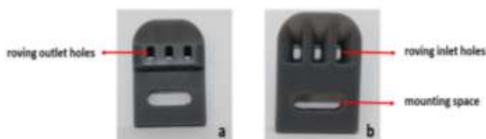
Figure 1. 3D printed three roving funnel a) front view b) back view
