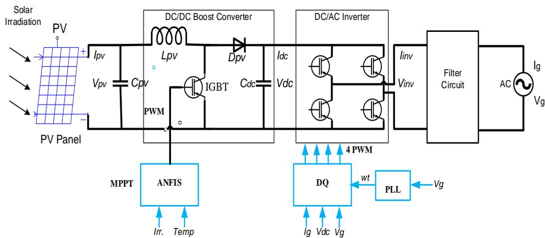
**Figure 1.** On-grid double stage single phase PV inverter with LCL filter.
