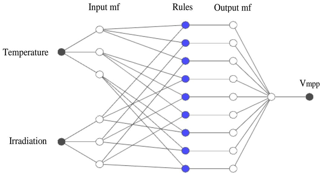
**Figure 7.** MPPT controller structure based on ANFIS.
