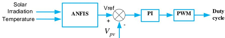
**Figure 4.** DC/DC boost converter control scheme based on ANFIS.
