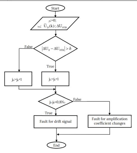
Fig.6. Algorithm flowchart representing determining the identify of drift or change in the transmission gain
