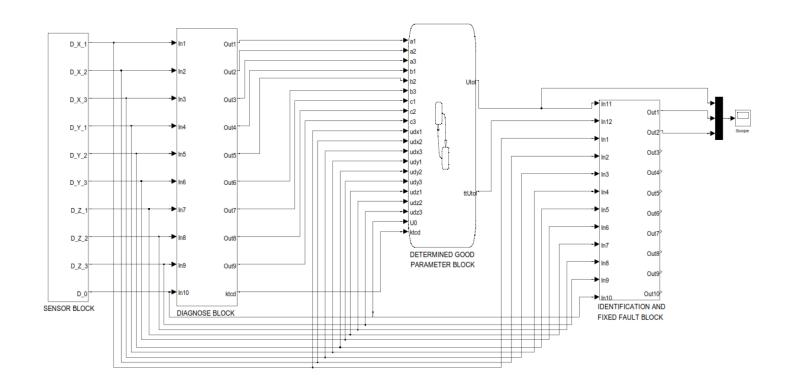
Fig 11. General simulation diagram for diagnosing, identifying and fixed fault of angular velocity sensors
