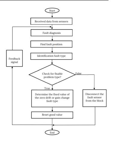
Fig.8. General algorithm flowchart representing fixed fault of sensors
