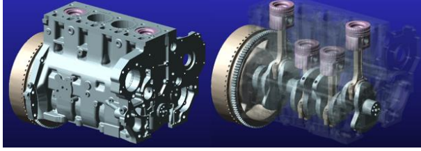
Şekil 11. Balansörsüz motor analizi-ADAMS (Without balancer engine analysis-ADAMS)
