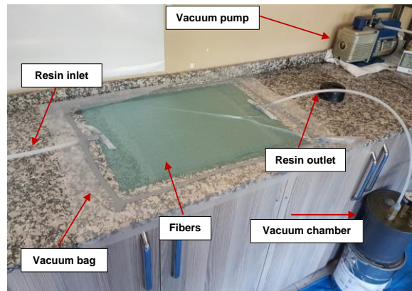
Figure 1. Vacuum infusion process setup
