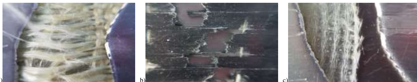
Figure 7. Fracture regions of Al layer composites a) Aramid Fiber Reinforced b) Carbon Fiber Reinforced c) Glass Fiber Reinforced
