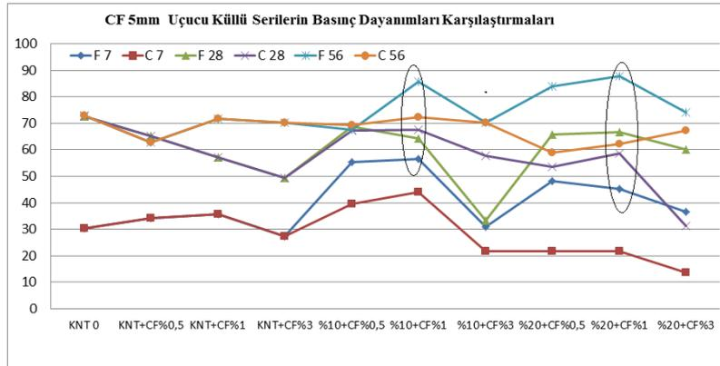
Fig. 11 Compressive strength values of Class F and C 5mm CF + fly ash samples
