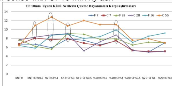
Fig. 10 Tensile Strength Values oClass F F and C 10mm CF + fly ash samples
