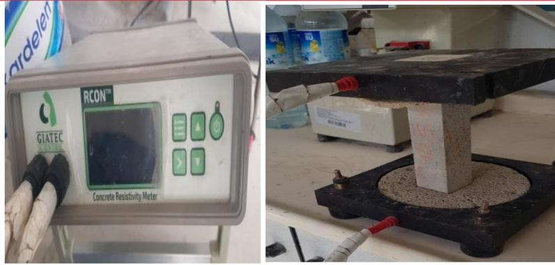
Fig. 4 Sample of which resistance measurement was carried out
