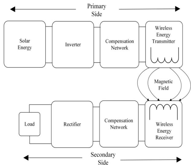
Figure 3. Solar energy-based IPT system.
