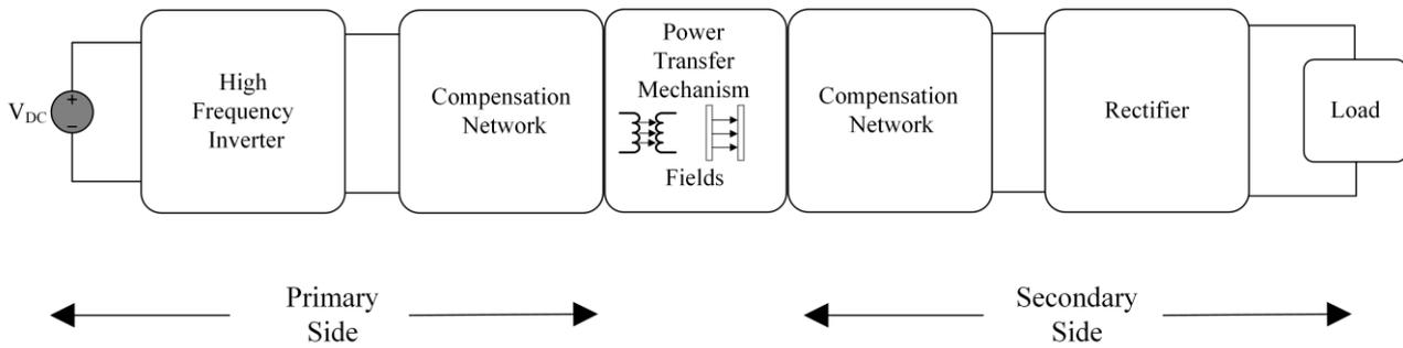
**Figure 2.** The typical configuration of a WPT system.
