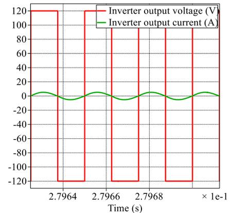
**Figure 6.** Inverter output voltage and current waveforms.
