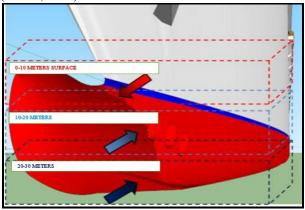
Fig. 4.The direction of the water column at Istanbul Strait and effects on the vessel.
