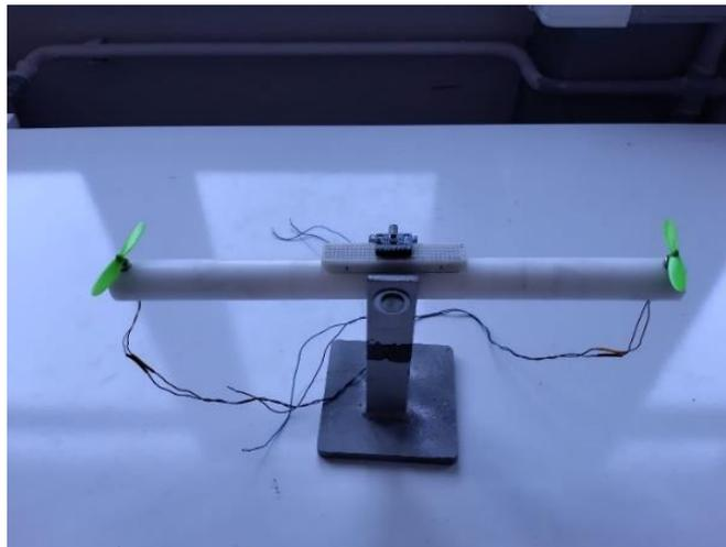
Figure 2. PID tester
