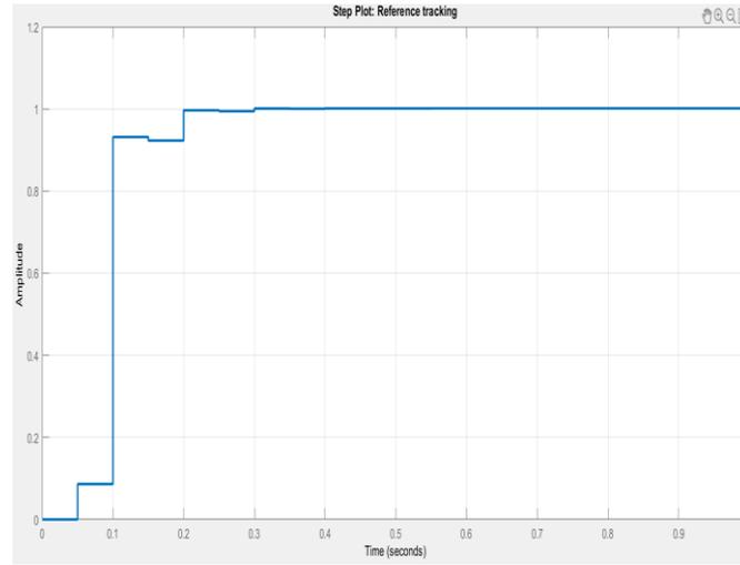
**Figure 7.** Simulation unit step response of the system
