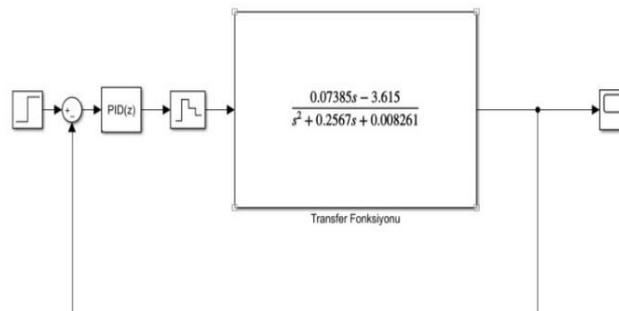
**Figure 6.** PID control block diagram
