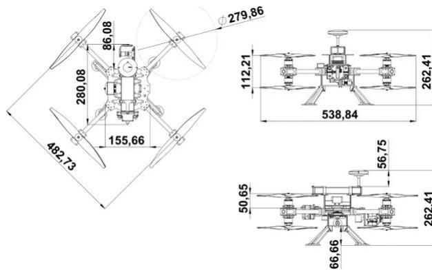
**Figure 1.** Dimensional parameters of the UAV
