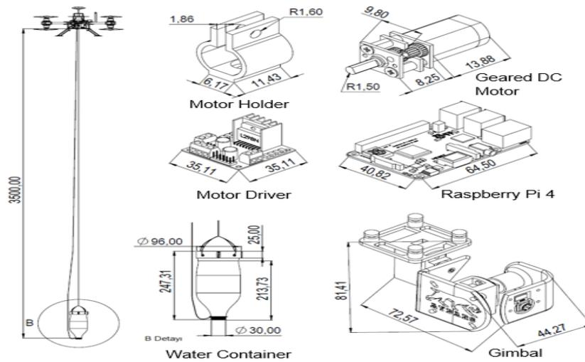
**Figure 7.** Technical details of the task mechanism and equipment
