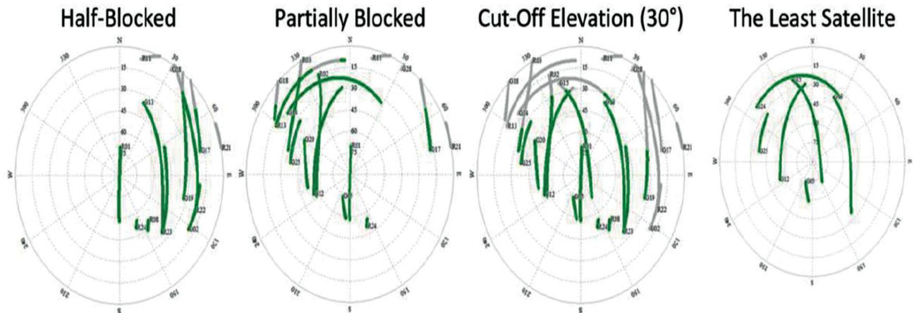
Figure 6. Variations on the satellite geometry.
