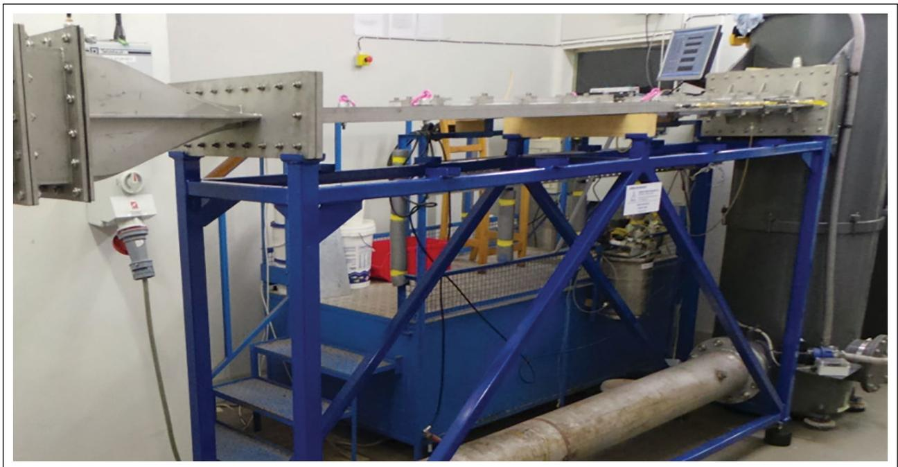
**Figure 2.** A view of the new test section of UNEW's flow cell.
