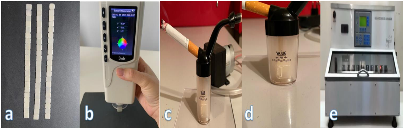
Figure 2: (a) prepared samples, (b) color measurement, (c) smoking chamber, (d) vertical sample inside the chamber and cigarette smoke, (e) tooth brushing simulator.
