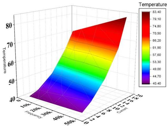
Fig. 5. Frequency-Current-Temperature graph for SCT20N120
