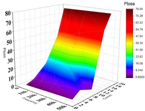
Fig. 6. Frequency-Current-Power loss graph for IRFP460
