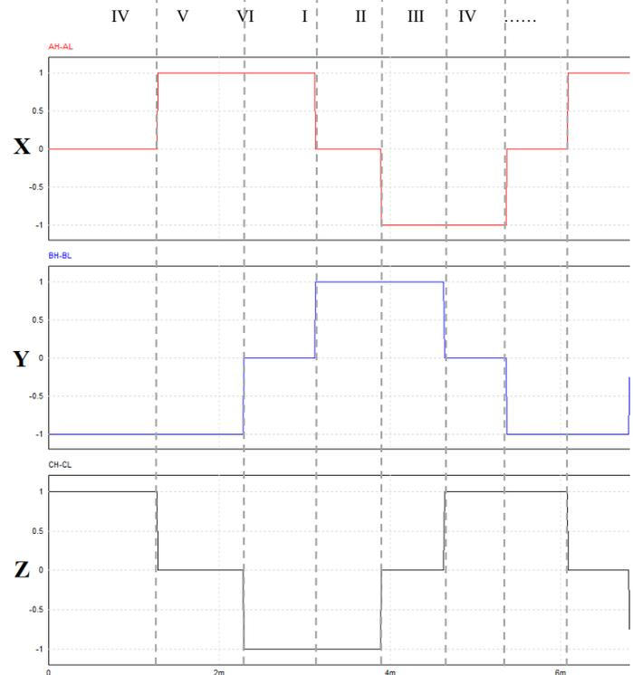
Fig. 2. Simulation of MOSFETS switching signals for inverter
