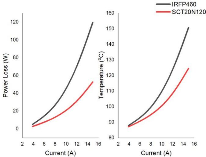
Fig. 10. MOSFET states at 85°C cooling temperature
