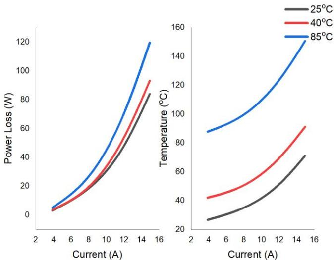
Fig. 11. IRFP460 values according to different cooling temperatures
