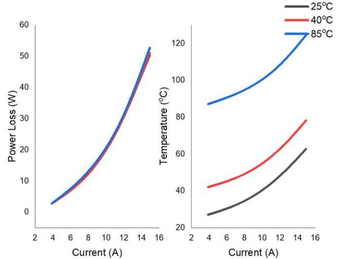
Fig. 12. SCT20N120 values according to different operating temperatures
