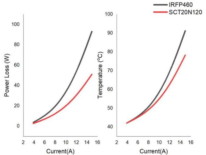
Fig. 9. MOSFET states at 40°C cooling temperature
