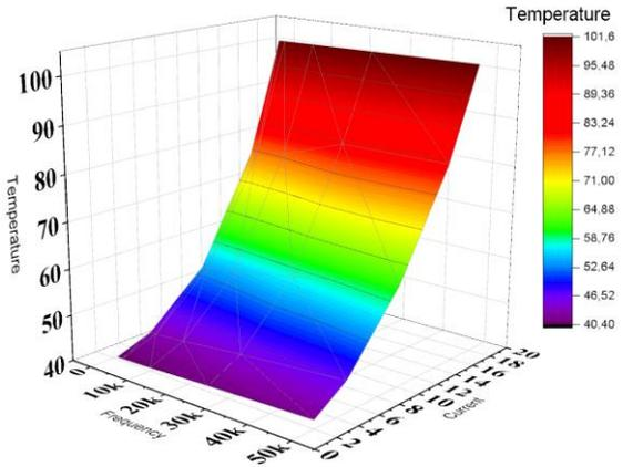
Fig. 4. Frequency-current-temperature graph for IRFP460
