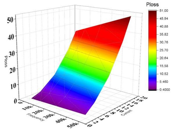
Fig. 7. Frequency-Current-Power Loss graph for SCT20N120
