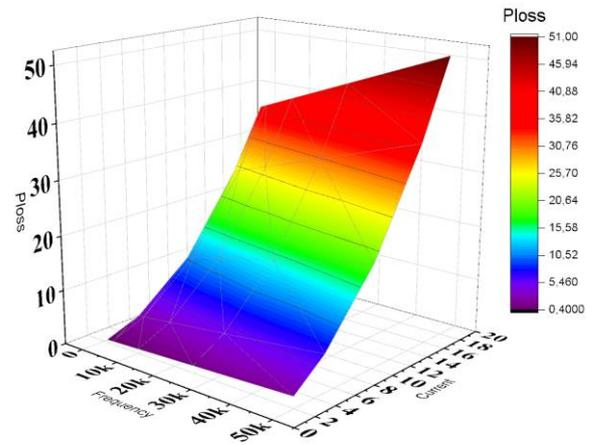
Fig. 7. Frequency-Current-Power Loss graph for SCT20N120
