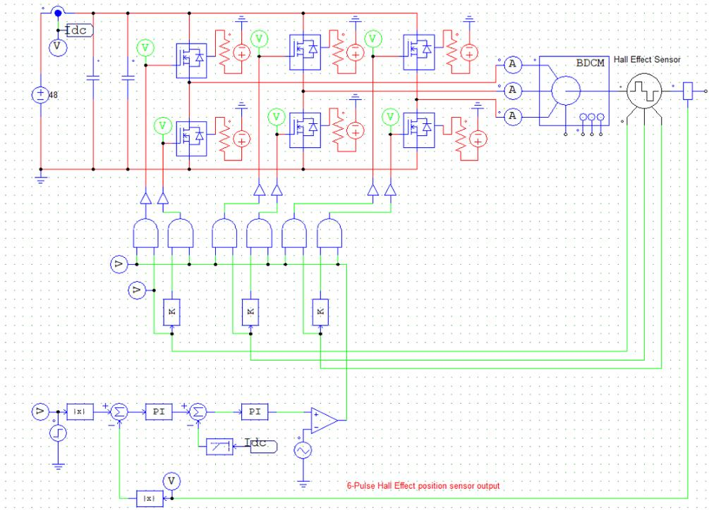
Fig. 1. PSIM Simulation Circuit.
