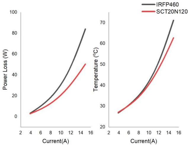
Fig. 8. MOSFET states at 25°C cooling temperature
