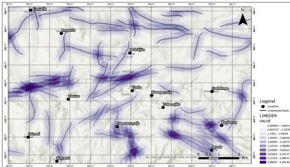
Figure 11. Fault (lineation) density in study area
